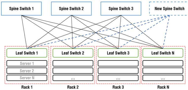
When a new Spine Switch is added, it requires the addition of a new physical connection to each existing leaf switch.
