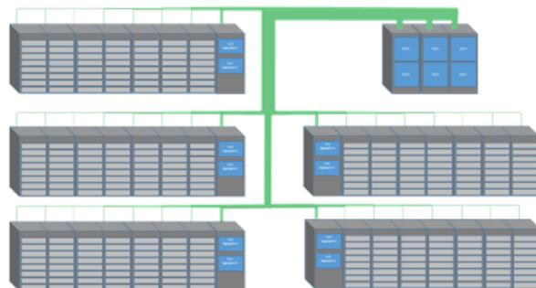
This aggregation reduced the volume of cabling going into the central switching rack. At the same time, data center operators started deploying cabling in a more structured manner, in order to simplify planning, installation and troubleshooting. Cables from servers were terminated on patch panels between devices, and cables were run between patch panels instead of direct point-to-point runs.
