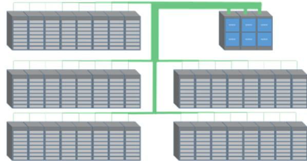
As connection density increased, the volume of cabling from each rack became too large to manage via this kind of direct cabling connections. It created operational issues and made troubleshooting connectivity in the thick web of cables on the switch side almost impossible, often causing outages for neighboring services.
