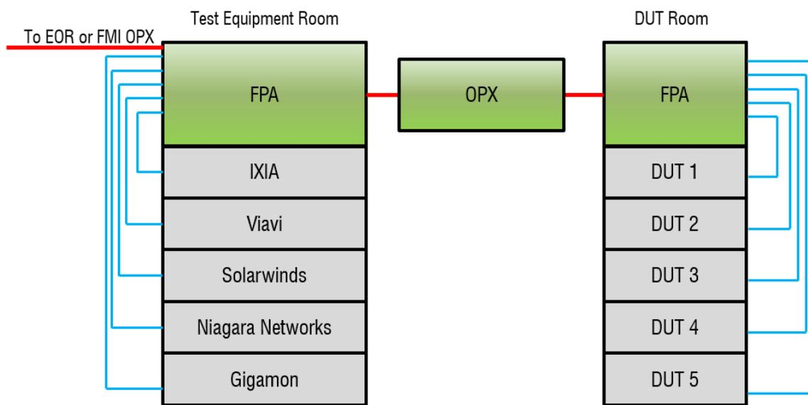
**Automated Connections:** The biggest benefit of The Glass Core<sup>™</sup> is the ability to automate connections via Fiber Mountain's orchestration software, All Path Director (APD). Through APD, any connection coming into an OPX can be configured to any port out, with the additional ability to multicast one "receive" port to up to 160 10G "transmit" ports in a single OPX.
